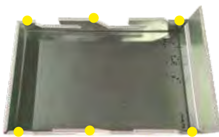
3. Folding the lateral edges and the triangular parts of the cassette to 90°.
